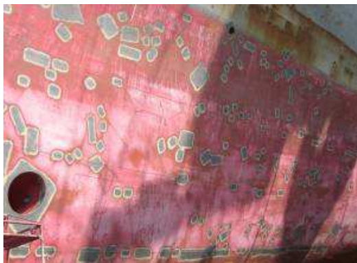
Square blast cleaning
