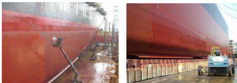
When spraying A/F paint, keep about 1m wide spray shift at right angle.
